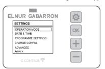
Use or to move up and down. Confirm with to enter the desired setting.
